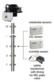
The KEL is an electrically controlled plate exhaust valve suitable for central ventilation systems with CRVB-N, CRHB-N and CTB Ecowatt Plus fans, which can be controlled e.g. by bathroom and toilet lighting, CO2 sensors, humidity sensors, thermostats, programmable time switches.
