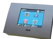
DR-CPhr programmable touch controller with LCD panel
